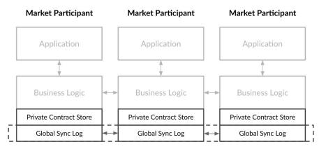
Figure 9. Including the two primary components of the Distributed Ledger Layer
