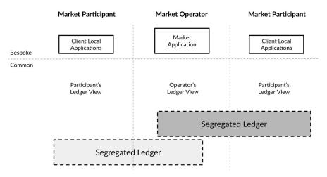
Figure 5. A Distributed Ledger with physically segregated ledgers
