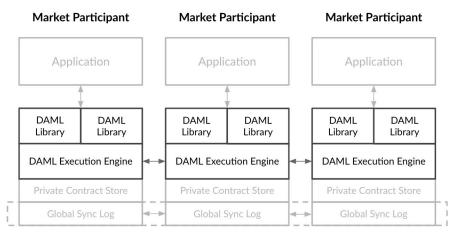
Figure 10. The two components of the Business Logic Layer
