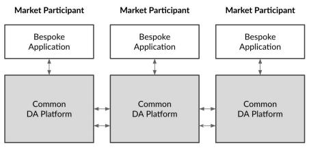
Figure 8. Applications are bespoke to the participant, but the Distributed Ledger Layer and Business Logic Layer of the DA Platform are common to all
